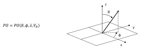
where  $\theta$  is the polar angle between the light exit direction and the normal vector to the surface, and  $\phi$  is the azimuth angle of the light exit direction as specified in the figure above.
