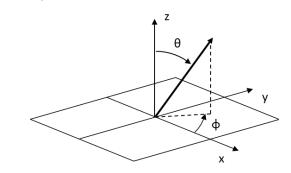
where  $\theta$  is the polar angle between the light exit direction and the normal vector to the surface, and  $\phi$  is the azimuth angle of the light exit direction as specified in the figure above.
