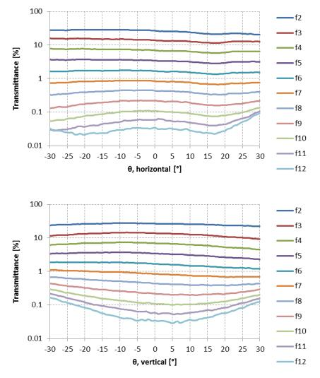
8.5. Angular transmittance PolarView®-ND(212) vs. FOS comparison
