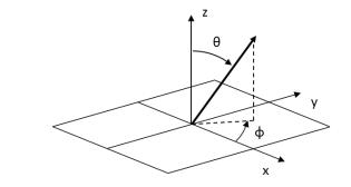
where  $\theta$  is the polar angle between the light exit direction and the normal vector to the surface, and  $\phi$  is the azimuth angle of the light exit direction as specified in the figure above.
