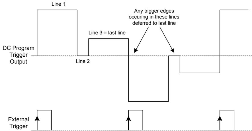
AC Line Trigger mode is supported in all versions of *LCDriver2* and with all LCC-230 device-side software. In AC Line Trigger, the time durations for each line are ignored, and the voltages of the lines of the program are held indefinitely until a trigger edge appears on the BNC connector. A rising trigger edge advances the program to the next line. At the last line of the program, execution wraps back to the first line.
