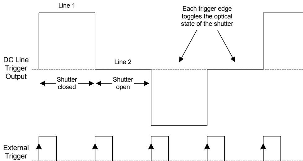
DC Line Trigger can also be used with PolarSpeed™ devices. Shown below is the cell #1 drive waveform in DC Line Trigger mode. The first line duration is set short and advances without a trigger edge; trigger edges advance lines 2 & 3, which are set by *LCDriver2* to maximum duration.
