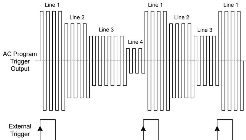
For DC programs, triggers occurring before the last line of the program are deferred until the last line is reached, and each external trigger toggles the polarity of the line voltages, as shown below. DC Program trigger is typically used to ‘sync’ (phase lock) the LCC-230 to an external periodic source (e.g. projector). For these applications, the last line’s duration should be “padded” by a couple ms to insure that the trigger edge will always fall within the last line.
