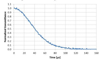
8.3. Closing time at room temperature, normalized transmittance vs. time
