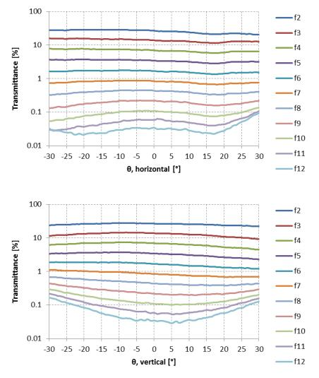
8.5. Angular transmittance PolarView®-ND vs. FOS comparison
