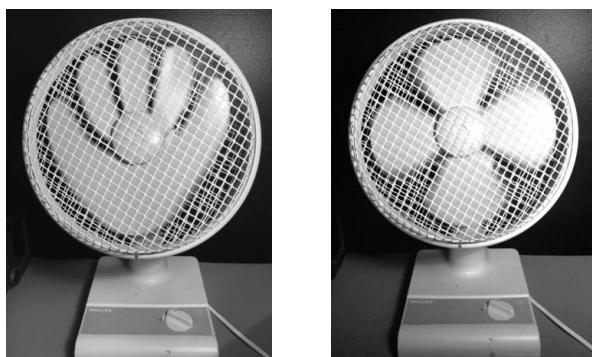
*Left: Image captured using a simple rolling shutter sensor. Right: Same sensor together with LC-Tec's X-FOS(G2)-CE-AR global shutter.*
