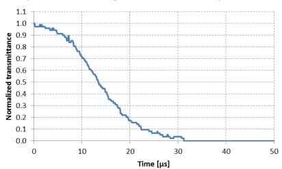
8.3. Closing time at room temperature, normalized transmittance vs. time (cell 2 drive voltage switched on at t=0)
