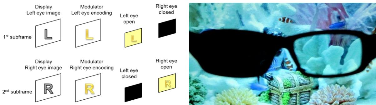
How the observer would see the display through a pair of passive circularly polarized viewing glasses during the right eye subframe.
